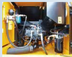
▲ Engine oil filter configuration is more efficient The filter can be replaced without go through under the body with better maintainability and safety.
