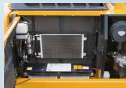
▲ Cooler The oil cooler and the intercooler and the radiator are arranged parallel to make the cooling effect better.
