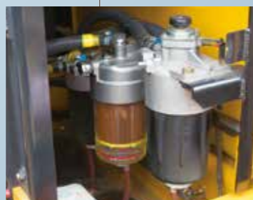
▲ Fuel filter By arranging the triple filters in the same position to improve the efficiency of replacement. Easy to access and improve safety.
