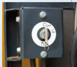
▲ Equipped with battery disconnect switch
