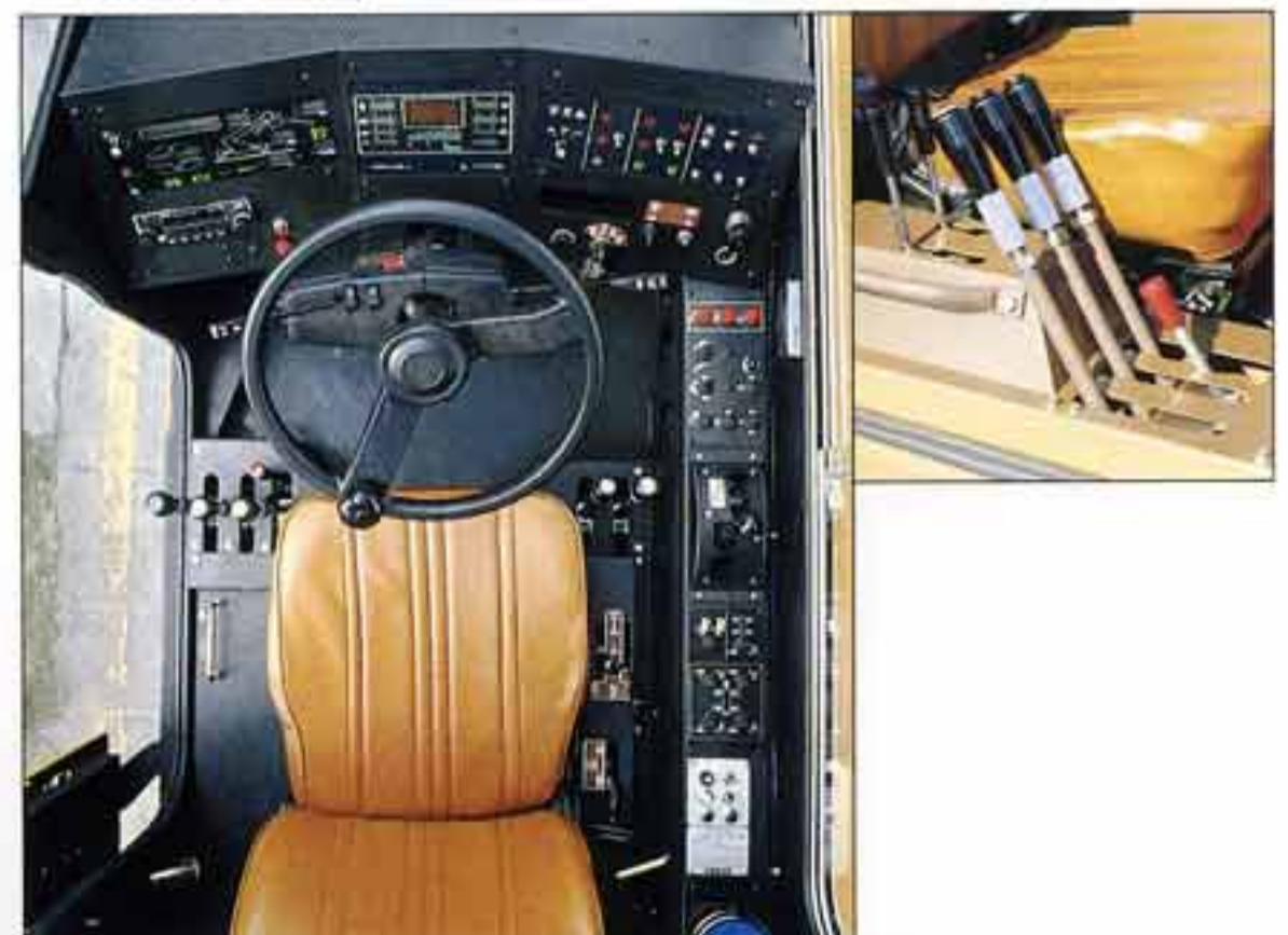
● Levers can be positioned to allow the operator easy access to the cab.
