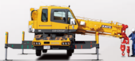
Set jib hook pin and connect the jib to boom top.
