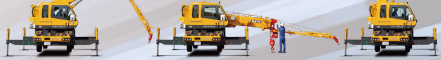
Hoist auxiliary hook to swing out the jib.
