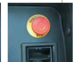
▲ Emergency engine stop switch (for crane operation)
