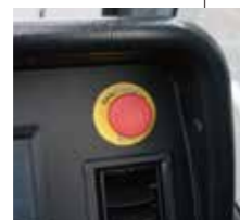
▲ Emergency engine stop switch (for crane operation)
