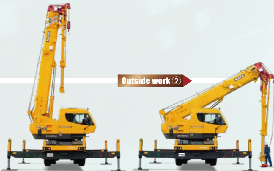
Extend the Boom and release the Jib.
