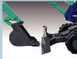
Closer proximity between bucket and dozer blade
