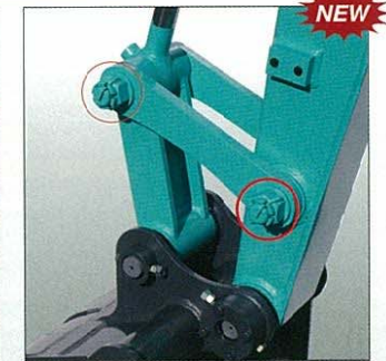
The arm-end and boom-arm joint are fixed with castle nuts. The reduction of horizontal tolerance is achieved.
