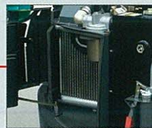
Radiator and Hydraulic fluid filter
