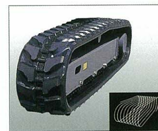
Like no others in the industry, the rubber shoe is warranted for either 2 years or 1,500 hours against steel cord cut-off. * See Page 27 for details.
