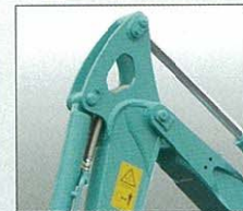
The arm-end and boom-arm joint are fixed with castle nuts. The reduction of horizontal tolerance is achieved.
