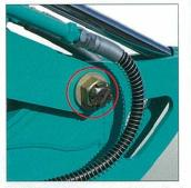
The arm-end and boom-arm joint are fixed with castle nuts. The reduction of horizontal
