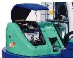
Inspection cover and tool box
