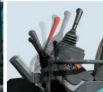
All operations are blocked when the lever is raised.
