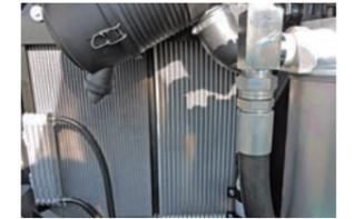
Suction type "side-by-side cooler" cleaning system
