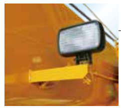
▲ Working light (boom)
